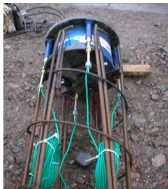
O-cell Assembly and Instrumentation.
